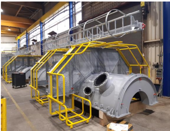
Mill Shell with maintenance platforms
