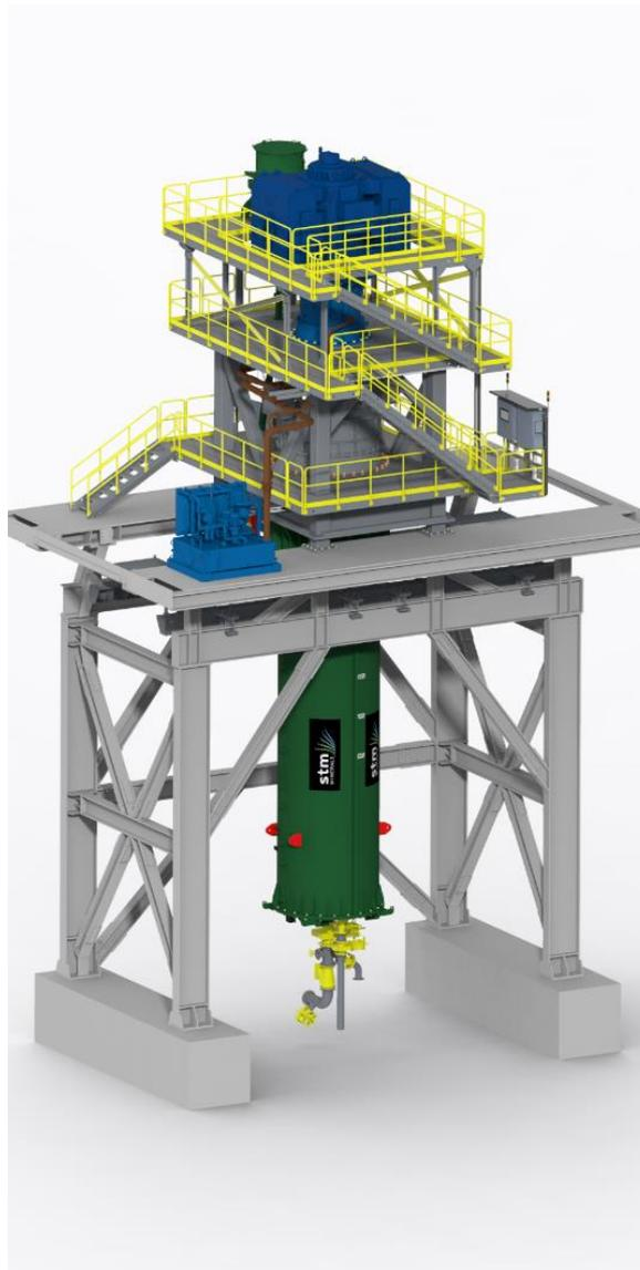
Schematic impression of a VRM mill
