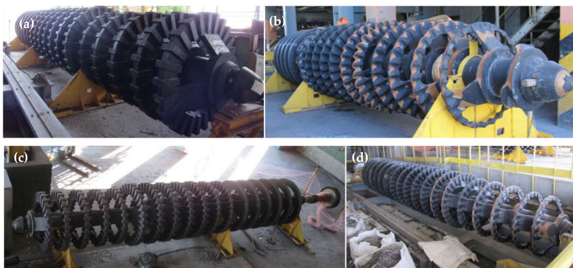
Figure 6 – New and Worn Rotors in Plant Trial Period
